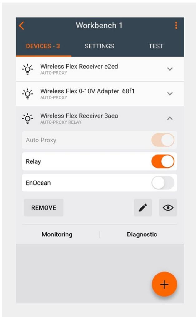
To configure a device as a Relay, toggle **Relay** in the Devices tab of the Zone view.
