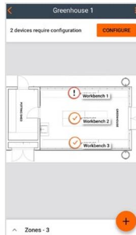
**HINT:** If the warning icon appears, tap that zone → open **DEVICES** tab → tap **CONFIGURE ALL**. The devices added to the zone should be automatically configured one by one.
