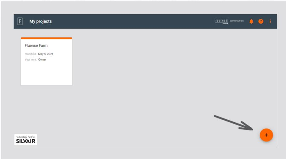
**Projects:** can represent a whole building, or single room or a floor for smaller installations. Each project is a single mesh network.
