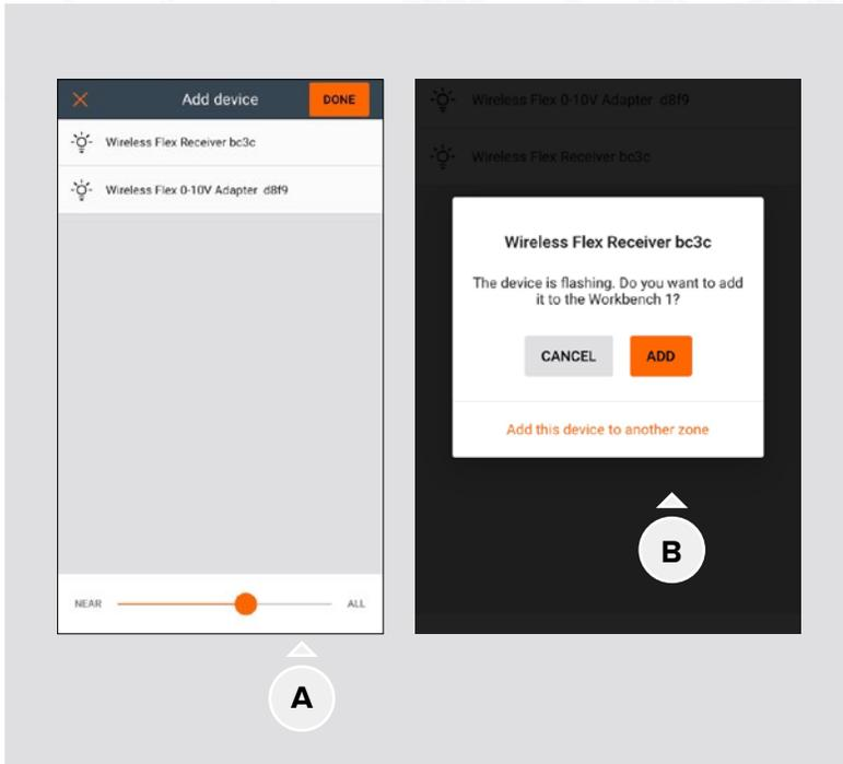
**A – Slider:** to reduce the number of available devices displayed, move the slider to the left. This filters them by signal strength and may be useful on large installations.
