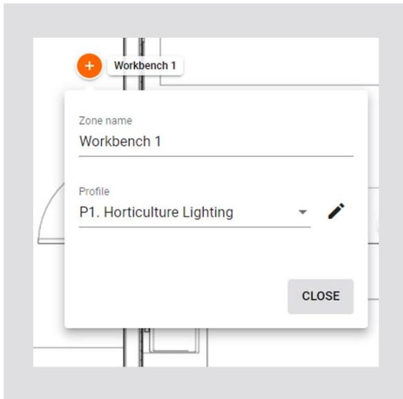
**Add the zone name.** A zone is a group of devices that are controlled together. Zones don't necessarily have to be a physical space (e.g., a room) as a room may contain one or more zones, e.g., multiple areas controlled separately. More than one zone can be added to the same plan.
