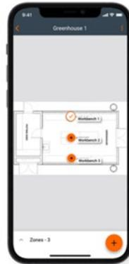
Prepare your commissioning plan off site, before anything is installed on site, by mapping the individual zones on a floorplan and defining lighting control profiles.
