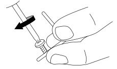
Insert the brackets into the channel windows on either end of the RAY fixture. Please ensure the screw-heads remain above the channel when inserting brackets.
