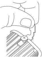
Slide brackets into desired position based on the support structure you are mounting to or hanging from. Ideal spacing should equal the distance from the center of the RAY fixture. When bracket is in desired position, hand-tighten the screws on each bracket to pin it in place.
