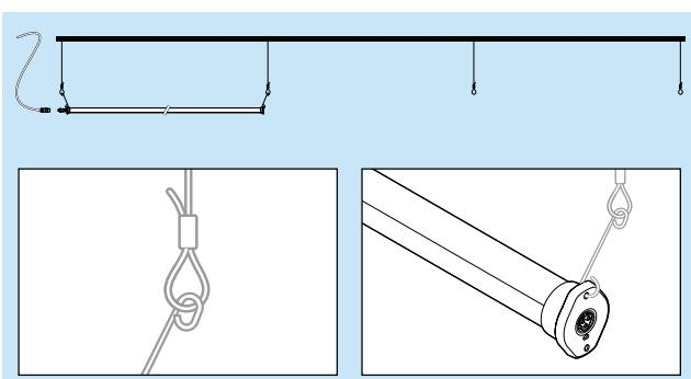
Hook up the other side of the first VYNE 2 module with the second mounting bracket around the loop of the second steel suspension cable.
